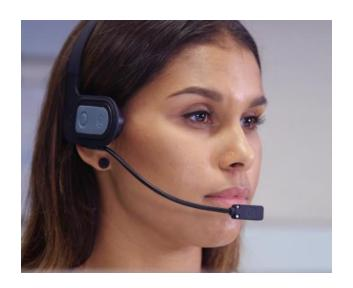
Quha Sento is the world's first contactless puff switch. It is used to perform a short mouse click or dragging together with the Quha Zono gyroscopic mouse.
